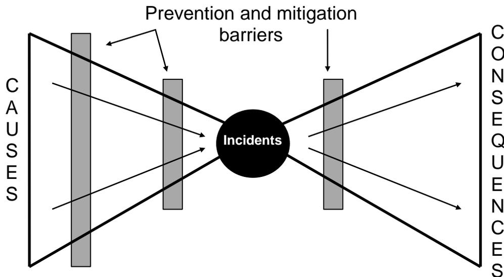
Figure 1-1: The cause/incident/consequence 'bow-tie' diagram
