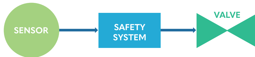
Figure 13. Safety instrumentation system with typical components
