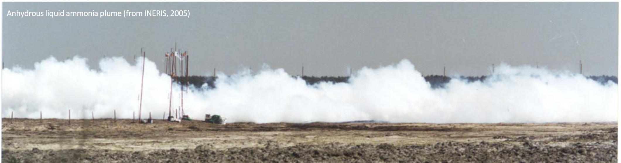
Anhydrous liquid ammonia leak
